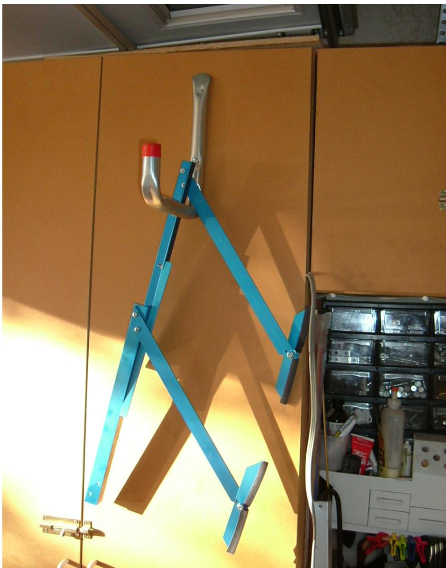
**To store the EZ Balancer, slightly loosen the nuts on the Cross Frame Member, then, using a Pantograph type of movement, push the Base Frame Members towards each other until they are touching.**
